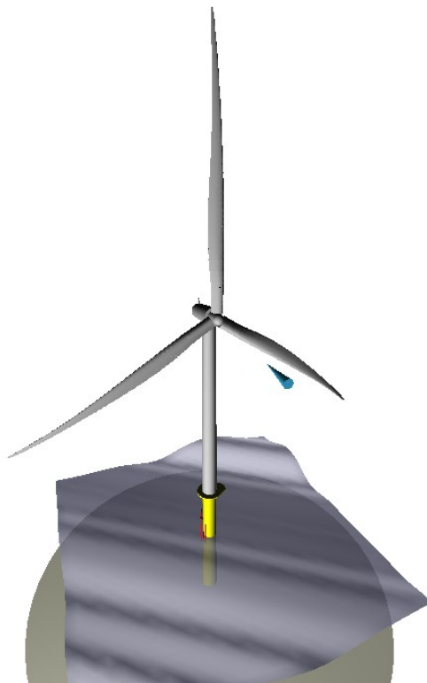
Figure 3-3: Illustration of a C2FLEX Simulation. The waves can be seen from a 30° direction compared to the turbine yaw direction.
